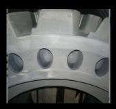
Beside the normal advantages of solid tires. WonRay skid steer tires with big and quite deep aperture holes on side. The big sizes aperture holes can only be made when the technology good enough to make sure the holes will not easy to broke during heavy load running.
